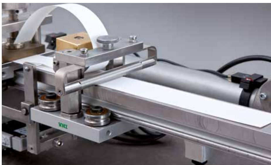
Setting speed test equipment in a WACKER laboratory.
