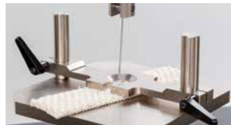
The tuft bind test examines how well the precoat adheres the fibers to the primary backing.
