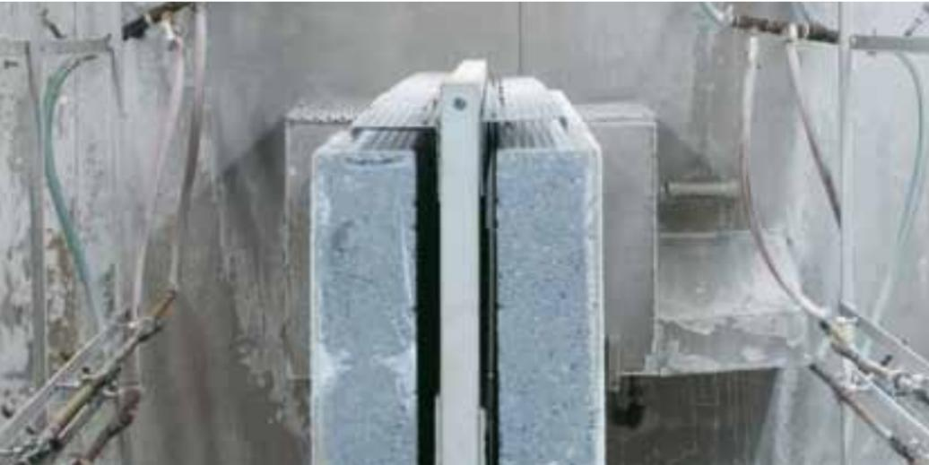
As one of few facilities in Europe, our Burghausen technical center boasts two EOTA climatic chambers in which we can simulate year-long weathering of walls in an accelerated process.
