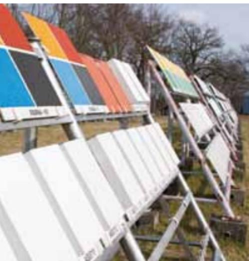
One example of an unusual test method is our outdoor weathering rig, which provides reliable long-term data on specific tile-adhesive formulations.
