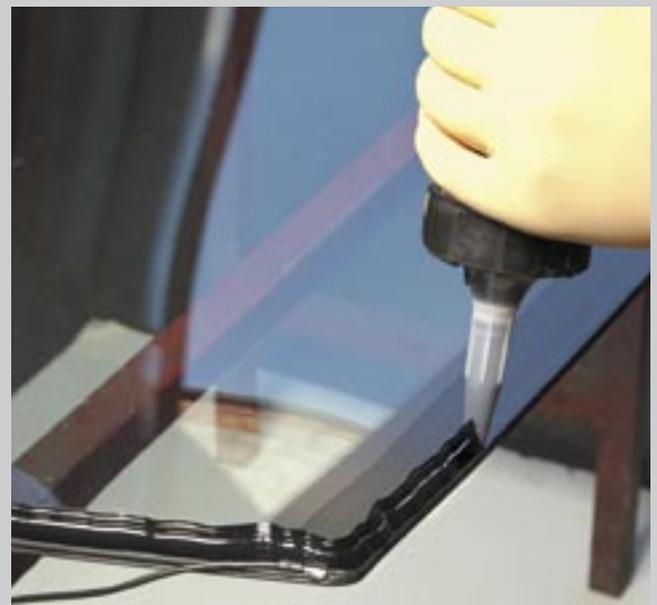
**Figures 1a and 1b: Bonding a car windshield in place. The elastic adhesive also helps to make the car body more rigid and simultaneously serves as a seal to keep out rainwater.**
