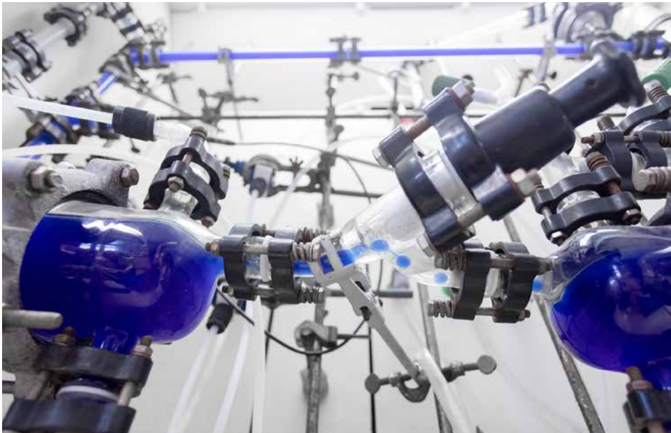
Glass circulating reactor: WACKER has developed a continuous manufacturing process for resin binders at a technical service lab at its Burghausen production site.
