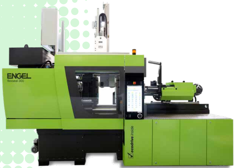
WACKER will use this Engel injection-molding machine at the K 2022 tradeshow to produce lemon presses from a biomethanol-based, food-grade silicone rubber.
