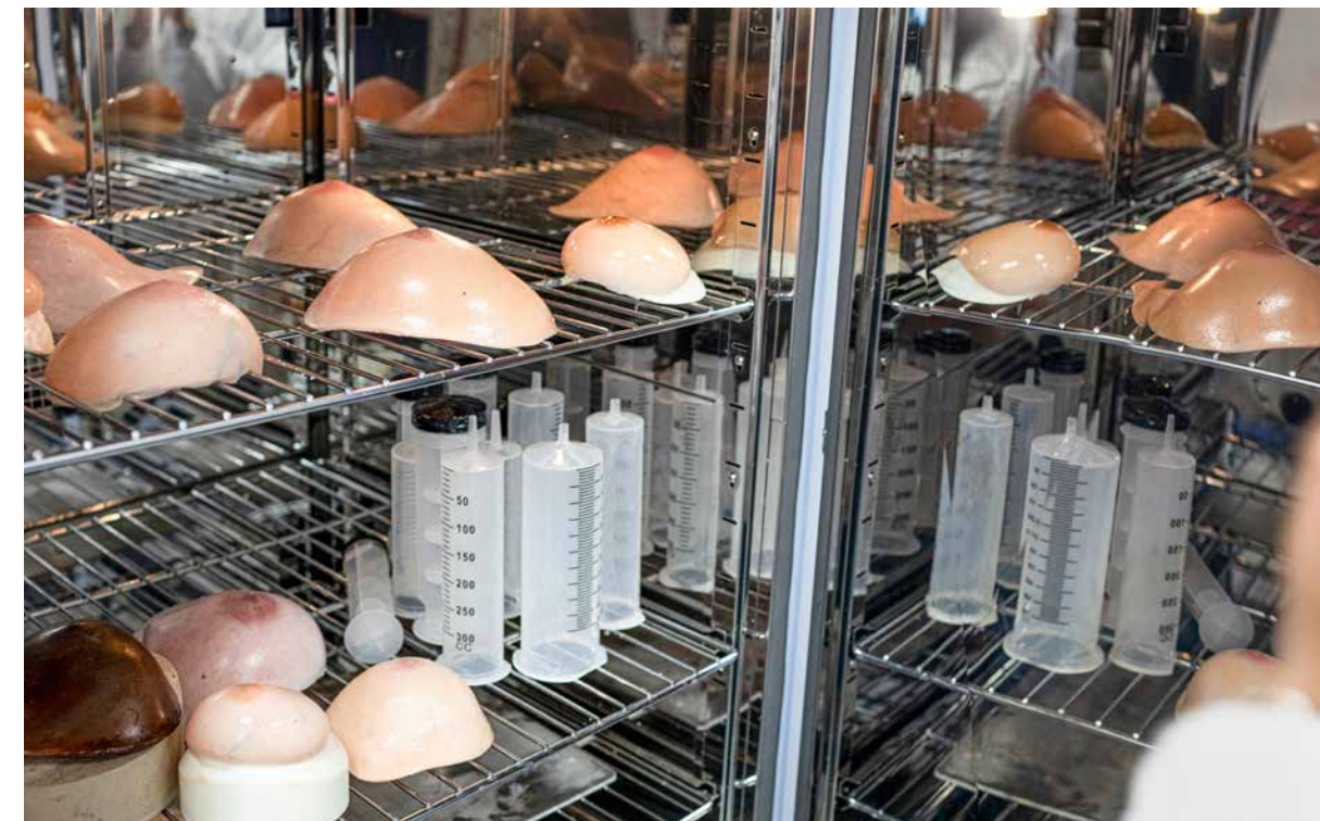
The individual parts of the prosthesis vulcanize in the drying oven.
