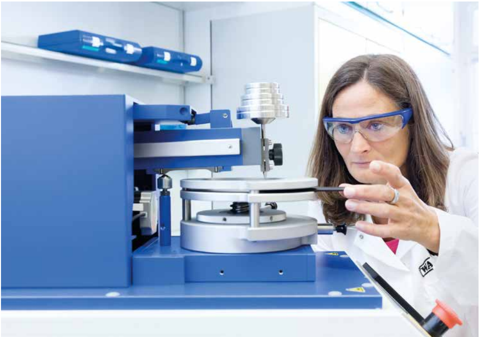
In the Erichsen scratch test, a needle moves at a specific force and speed across the plastic being tested, creating a grid pattern of scratches. The scratches are then examined closely and the color differences determined with a colorimeter.
