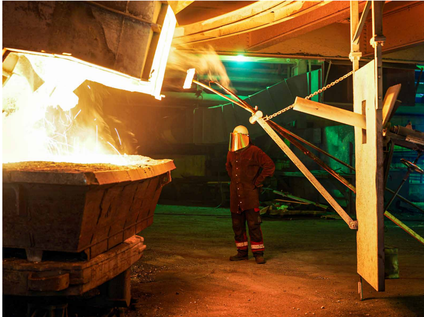
WACKER has been producing silicon in Holla, Norway, since 2010 – from quartz and coal at 2,000 °C.
