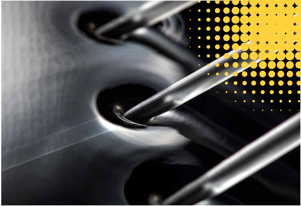
Preliminary stage for the production of blown or cast film: transparent pellet stock is made from a bioplastic and VINNEX® 2526. During this process, the strands pass through a water bath.
