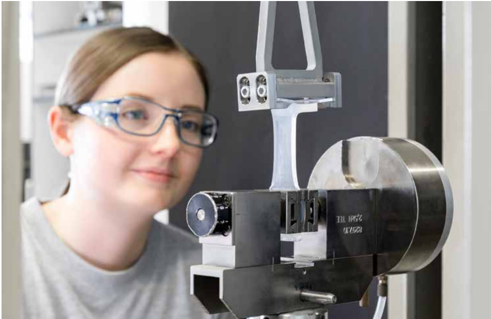
Peel testing stresses samples of multicomponent materials to their breaking point. In samples made of ELASTOSIL® LR 3078 and polycarbonate, it was the soft silicone component which consistently tore. The bond between the hard and soft components remained intact.
