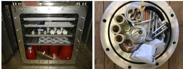
Examples of gas chambers / pressure containers for aging tests [8]
