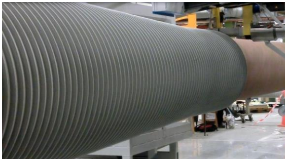
HTV silicone extrusion – joint free housing
