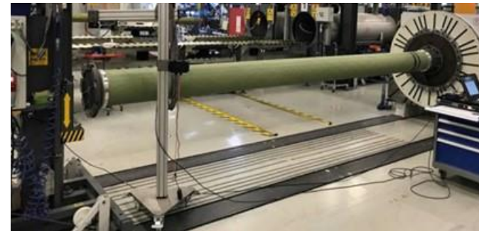
Routine bend & pressure/ tightness test.
