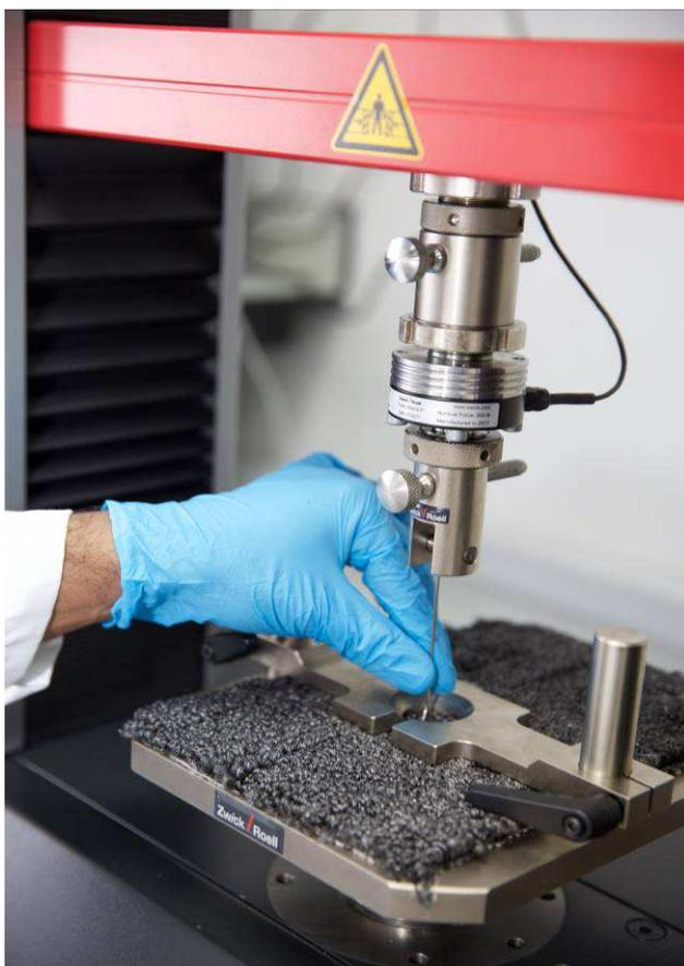
In the new polymers lab, WACKER experts are testing formulations with VAE dispersions as a binder in tufted carpet backing applications (photo: Wacker Chemie AG).
