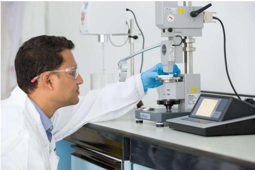
WACKER's lab for silicone elastomers in Dubai: A technical manager is performing a shore hardness test. In the MEA region, silicone elastomers are increasingly used in growing industries such as energy and mold making (photo: Wacker Chemie AG).
