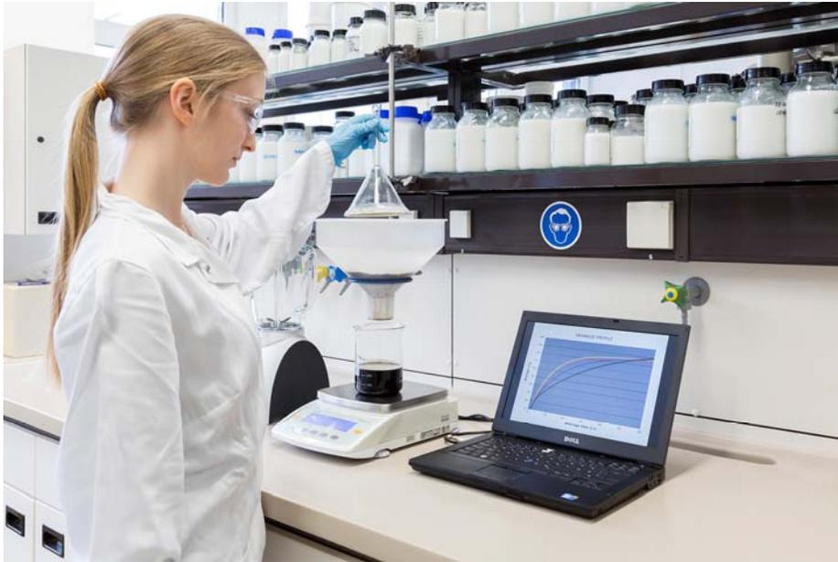
The rate at which pulp slurry is dewatered can be measured in drainage tests. WACKER's new silicone tensid PULPSIL<sup>®</sup> 968 S accelerates dewatering to unprecedented levels and improves the washing process during pulp making significantly. (Photo: Wacker Chemie AG)
