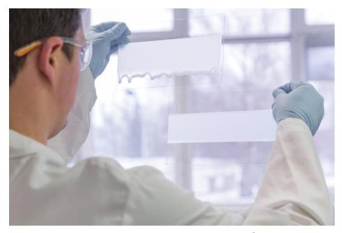
Industrial adhesives formulated with WACKER's HDK® H21 pyrogenic silica are extremely resistant to sagging and do not run on sloping or curved bonding surfaces. (Photo: WACKER Chemie AG)
