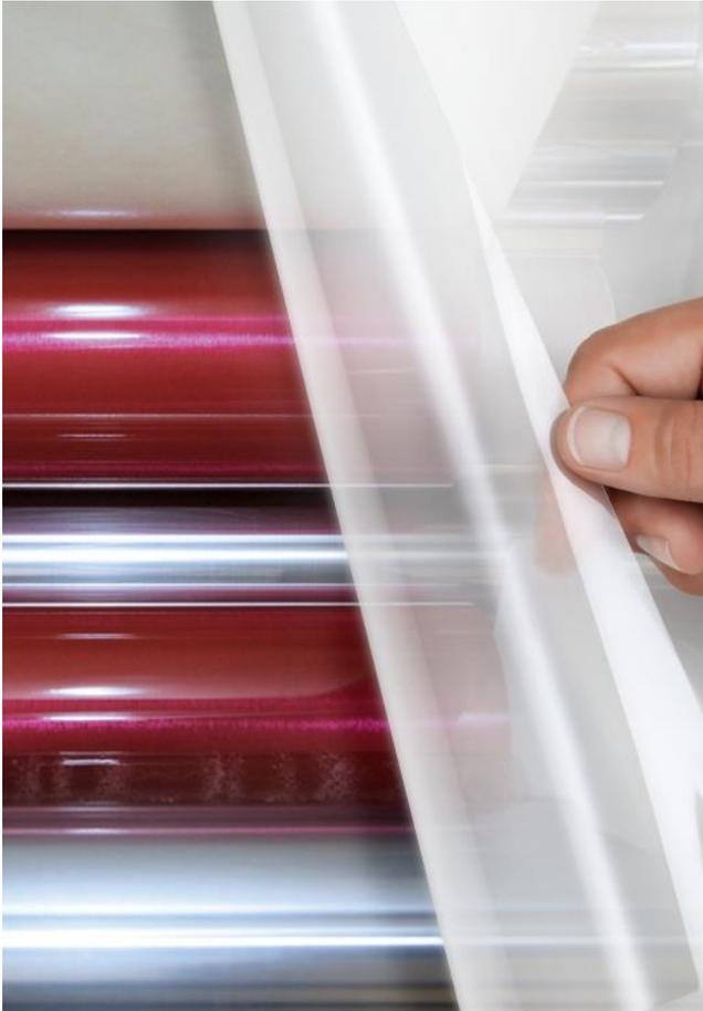
WACKER's new DEHESIVE® PSA 84X solvent-based silicone pressure adhesive (PSA) series consists of three products. They feature low, medium and high adhesion force respectively. The desired adhesion range can also be realized by cold blending. (Photo: WACKER)
