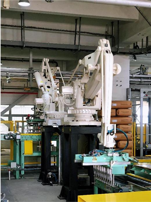
After the improvement project, WACKER's HDK<sup>®</sup> packaging station realized fully automated manufacturing process, including palletizing by robot. (Photo: WACKER)
