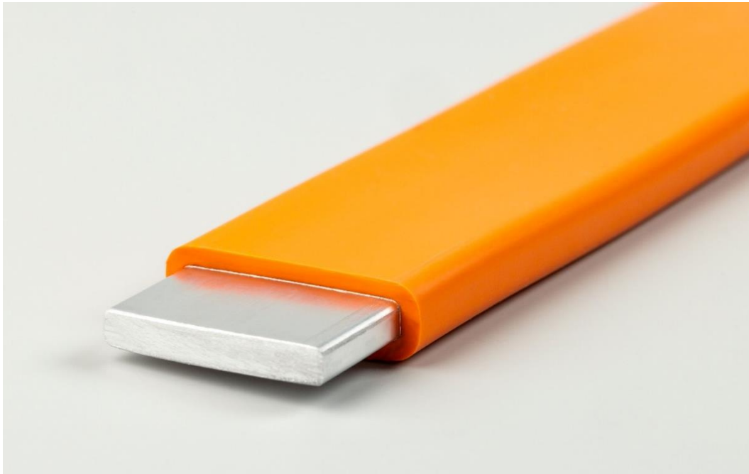
Busbar insulated with ELASTOSIL® R 531/60. The bar is bent and fit into the battery architecture after sheathing. Thanks to its high elasticity and notch impact strength, the silicone can easily cope with this molding and bending process. (Photo: WACKER)
