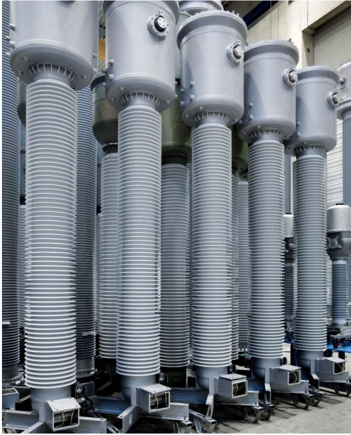
POWERSIL® 1900 A/B, WACKER's new high-consistency silicone rubber, facilitates the low-cost, high precision production of composite hollow-core-insulators via spiral extrusion processes. (Photo: WACKER)
