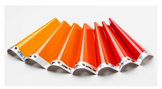
Metal sheets after a conical bending test. Thanks to the flexibility of SILRES® HP 2000 LV, the pigmented epoxy-polysiloxane topcoat remains crack-free. WACKER will be premiering the hardener at European Coatings Show. (Photo: WACKER).
