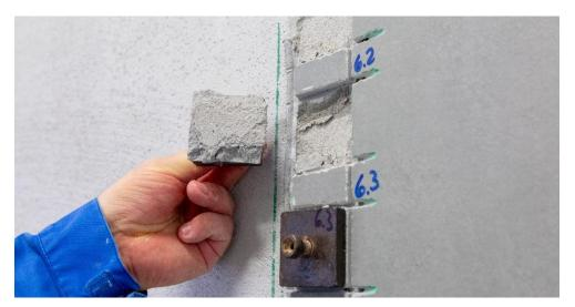
In tile adhesive formulations with CEM II and VINNAPAS® 8118 E, 8620 E or 7220 E, which contain water-repellent monomers in a terpolymer, the tensile adhesion strength following immersion in water is significantly improved and the requirements specified in the standard are thus met. (photo: WACKER)
