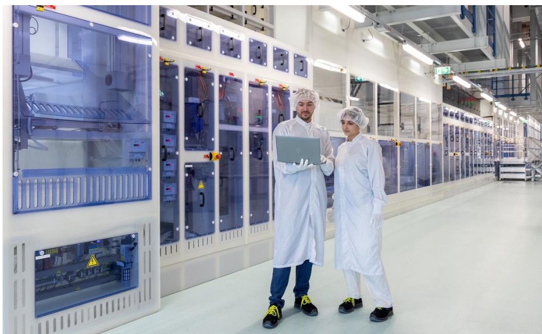
View of the Etching Line Next production facility. Acids are used to clean the polysilicon chunks before they are ready to be shipped to semiconductor customers across the world. (Photo: Wacker Chemie AG)
