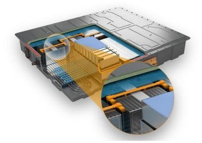
Interior view of a traction battery in an electric vehicle. The enlarged section shows the busbar (orange) insulated with ELASTOSIL® R 531/60. It is bent and fit into the battery architecture after sheathing. Thanks to its high elasticity and notch impact strength, the silicone can easily cope with this molding and bending process. (Graphic: WACKER)
