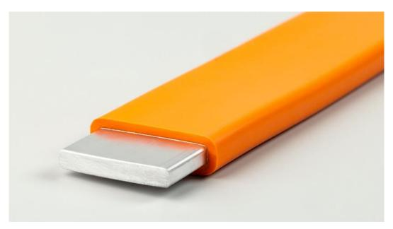
Busbar insulated with ELASTOSIL® R 531/60 (orange). The new silicone rubber ceramifies in the event of a fire. As a result, the rails remain insulated even in the event of an accident or vehicle fire. This provides additional protection to passengers of electric vehicles and rescue workers. (Photo: WACKER)
