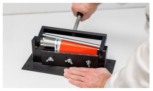
Testing the flexibility of an epoxy-polysiloxane topcoat in the mandrel bending test. The coating is based on the SILRES® HP 2000 LV hardener, which WACKER will present for the first time at ECS 2025. (Photo: WACKER).
