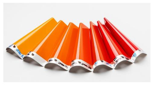
Metal sheets after a conical bending test. Thanks to the flexibility of SILRES® HP 2000 LV, the pigmented epoxy-polysiloxane topcoat remains crack-free. WACKER will be premiering the hardener at ECS 2025. (Photo: WACKER).
