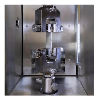
Crack-bridging test according to EN 14891: Waterproofing membranes formulated with VINNAPAS® 754 ED and VINNAPAS® 764 ED can compensate for cracks even at temperatures below freezing, thus reliably protecting the building from water penetration. (Photo: WACKER)
