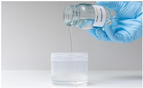
Celebrates its premiere at ECS 2023: SILRES® IC 900. This silicone resin was developed as a binder for solvent-based paints and coatings that have to withstand high temperatures. The product can even be used for formulating high-solids coatings. (Photo: WACKER)
