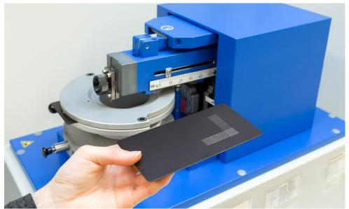
At ECS 2023, WACKER will be presenting a novel silicone resin for heat-resistant, water-based coating formulations. Cross-cut tests show that the adhesive properties of SILRES® M 51 E are similar to those of high-temperature paints and coatings formulated with solvent-based silicone resin binders. (Photo: WACKER)
