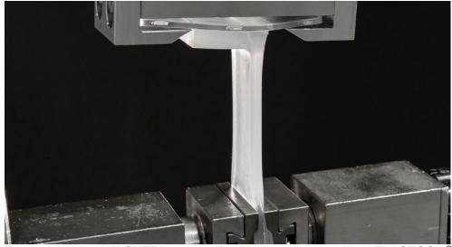
Tests show that WACKER's new self-adhesive silicone rubber ELASTOSIL® LR 3078 adheres excellently to polycarbonate without pretreatment. This makes efficient large-scale production of polycarbonate-silicone combinations possible, for example in medical technology. (Photo: WACKER)
