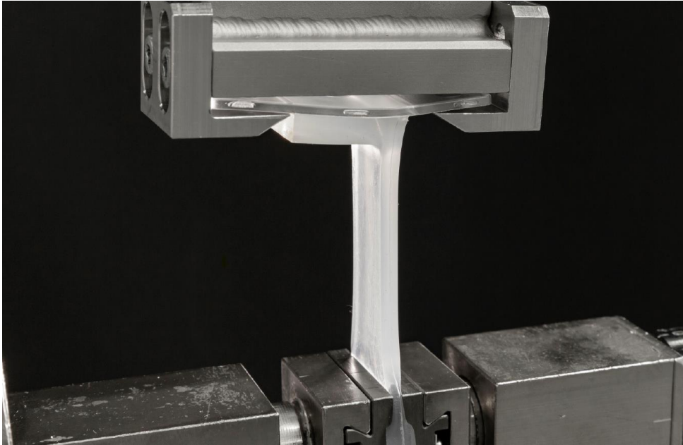
Adhesion tests show that WACKER's new self-adhesive silicone rubber ELASTOSIL® LR 3078 adheres firmly to polycarbonate without pretreatment. (photo: WACKER)
