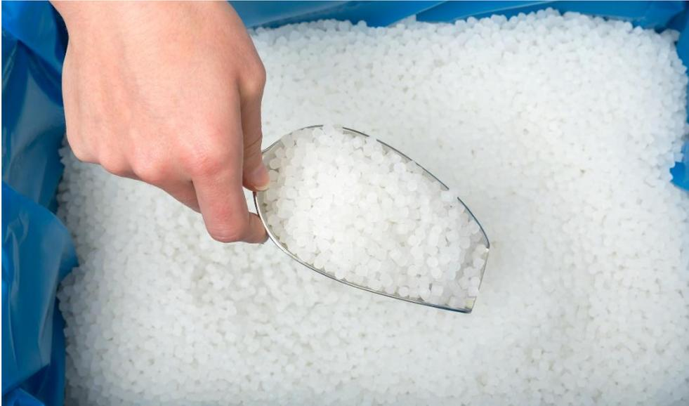
WACKER will present a new silicone-based additive masterbatch for polyethylene compounding at K 2022. GENIOPLAST® PE50S08 makes it easier to manufacture ready-to-use polyethylene molding compounds and improves the surface properties of the resulting plastic products. (Photo: WACKER)
