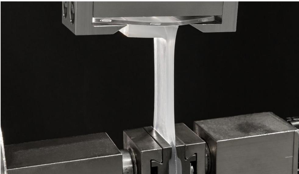
Tests show that the new self-adhesive silicone rubber ELASTOSIL® LR 3078 from chemical group WACKER adheres excellently to polycarbonate without pretreatment. This makes efficient large-scale production of hybrid parts possible, for example in medical technology. (Photo: WACKER)
