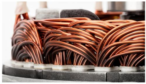
WACKER's new SILRES® H60 silicone resin was specifically developed for the trickle impregnation of electric motors. Introduced at this year's CWIEME, the resin is resistant to high temperatures and makes it possible to rapidly impregnate coil windings. (Photo: WACKER)
