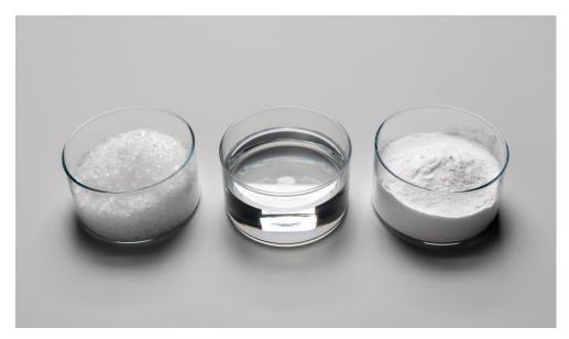
At CWIEME Berlin, WACKER is presenting flame retardant silicone resins for electrical engineering applications. SILRES® silicone resins are available as flakes (SILRES® MK FLAKES), liquids (in this case: SILRES® H60) and powders (SILRES® MK POWDER, SILRES® H 44). (Photo: WACKER)
