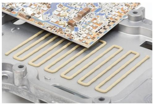
Thermally conductive silicone gap fillers from WACKER optimize the thermal transport between an electronic circuit that becomes hot during operation and the heat sink. With the successful certification according to standard IATF 16949, the Munich-based chemical Group WACKER can directly supply automobile manufacturers as well as system and module suppliers. (Photo: WACKER)
