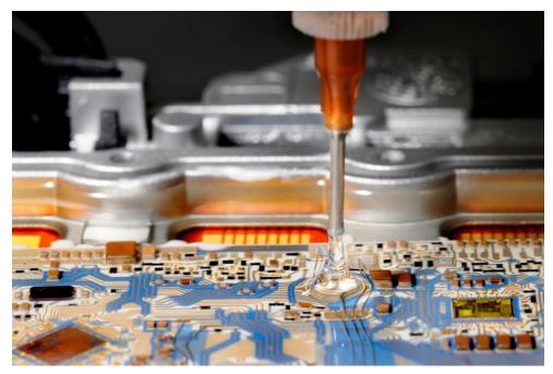
WACKER's silicone gels were especially developed for manufacturers of electronic components. Particular products can be cured at room temperature or elevated temperatures. Gels with rapid curing through UV-radiation are also available. (Photo: WACKER)
