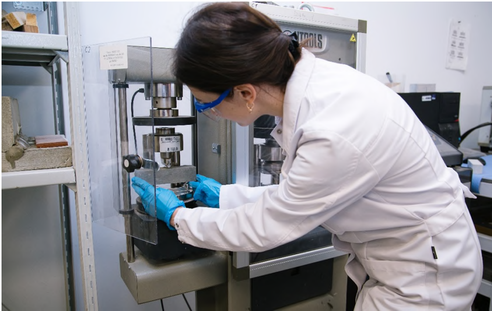
Mechanical pressure tests are among the services that the new laboratory in Moscow offers for water-repellent treatment of cement and concrete. These analyses provide insight into the strength of concrete formulations. (Photo: WACKER)
