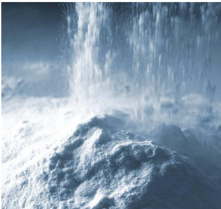
VINNAPAS® dispersible polymer powder. It enhances key properties of cementitious construction materials such as tile adhesives and grouts, skimcoats, concrete and sealing slurries. (photo: WACKER)
