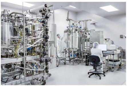
As a CDMO, Wacker Biotech US Inc. operates a specialized fermentation line with a capacity of 500 liters for the production and purification of pDNA (Photo: WACKER).
