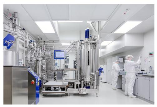
View of production at Wacker Biotech GmbH in Jena: modified *E. coli* bacteria are used to produce pharmaceutical proteins in fermenters. (Photo: WACKER)
