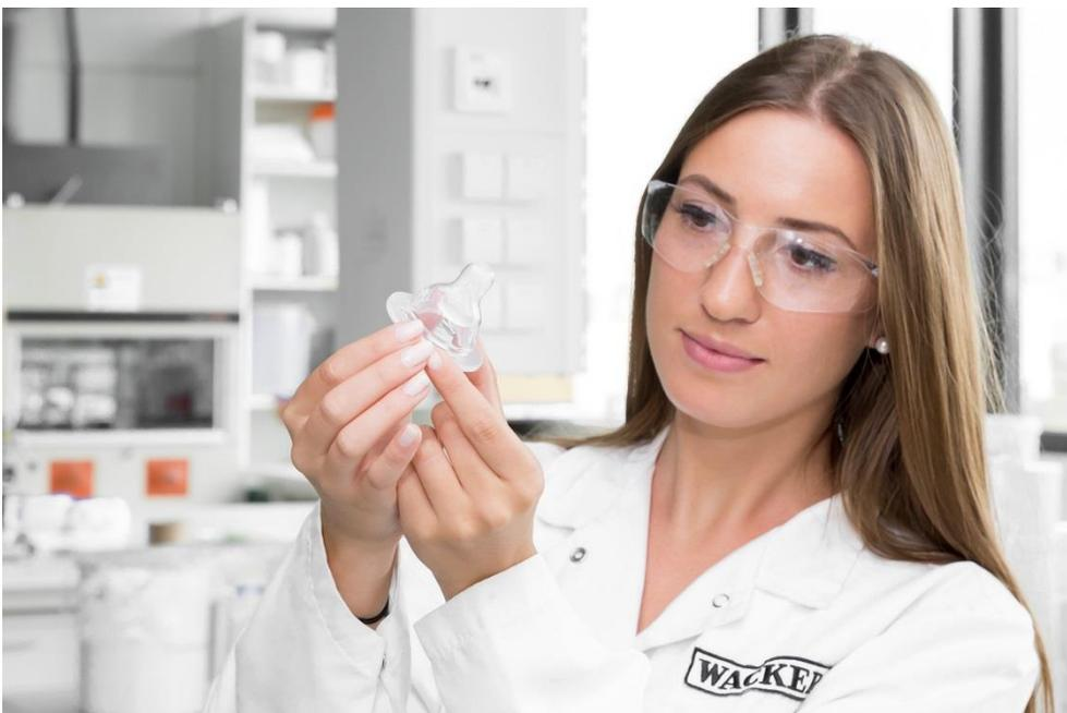
The new liquid silicone line ELASTOSIL® LR 5040 has been specially developed for applications in the baby-care, food-contact and medical industries. Its products contain only few volatile components and exhibit excellent mechanical properties even without thermal post-curing.
