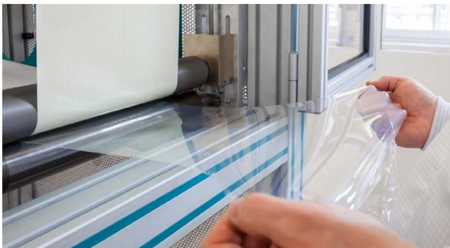
ELASTOSIL® Film is one of the more recent innovations from Munich-based chemicals group WACKER. This precision film, made from silicone, is thinner than a human hair, extremely flexible and durable. The continuous film lends itself to numerous applications, including sensors, actuators and energy-saving electrical relays. (Photo: Wacker Chemie AG).
