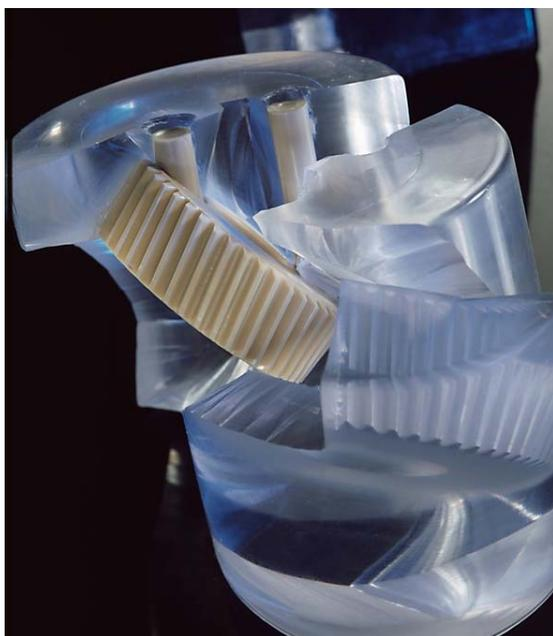
Mold-making compounds made from ELASTOSIL® silicone rubber are flowable, durable and easy to process. They cure to elastomers that possess excellent self-release properties and good transparency. ELASTOSIL® therefore meets all the key requirements on products used for prototyping, where high-volume, economical production is essential. (Photo: Wacker Chemie AG).
