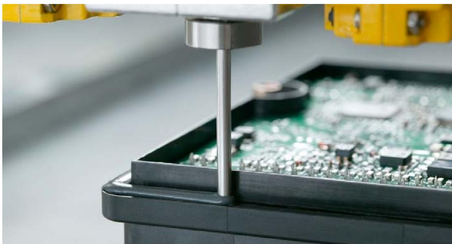
In the production of electronic controllers and sensors, ELASTOSIL<sup>®</sup> silicones seal housing components, bond individual elements and encapsulate electronic parts. Specialty ELASTOSIL<sup>®</sup> grades are particularly stable to automotive fuels and oils. (Photo: Wacker Chemie AG).
