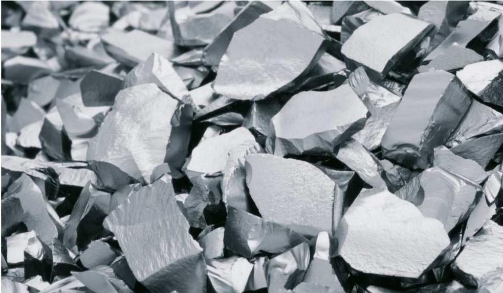
Polycrystalline silicon from WACKER, the Munich-based chemical company. The ultrapure material is used to produce silicon wafers for the solar and computer industries. (Photo: WACKER)
