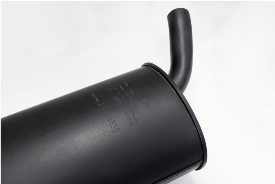
SILRES® REN70-M is a highly heat-resistant binder, making it suitable for coating mufflers, engine parts, stoves or incinerators (photo: Wacker Chemie AG).
