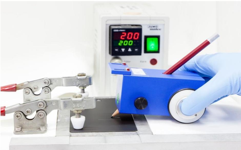
To ensure that coatings with SILRES<sup>®</sup> IC235 as binder also have sufficient surface hardness, pencil hardness tests are performed in the WACKER lab (photo: Wacker Chemie AG).
