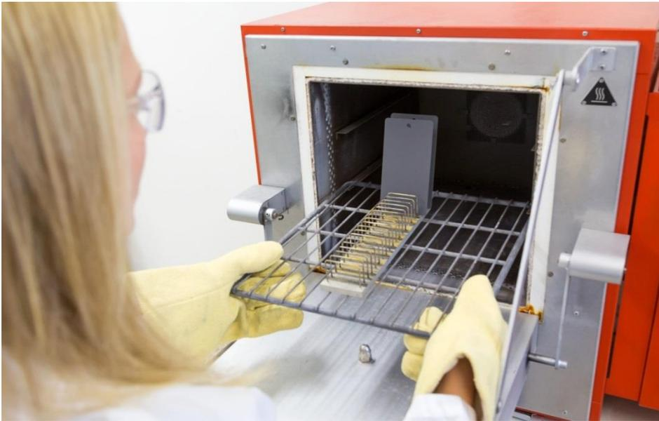
The thermal resistance of the new binder SILRES<sup>®</sup> REN70-M is tested in the WACKER lab by coating steel disks with a paint containing the binder and heating them up to 650°C (photo: Wacker Chemie AG).
