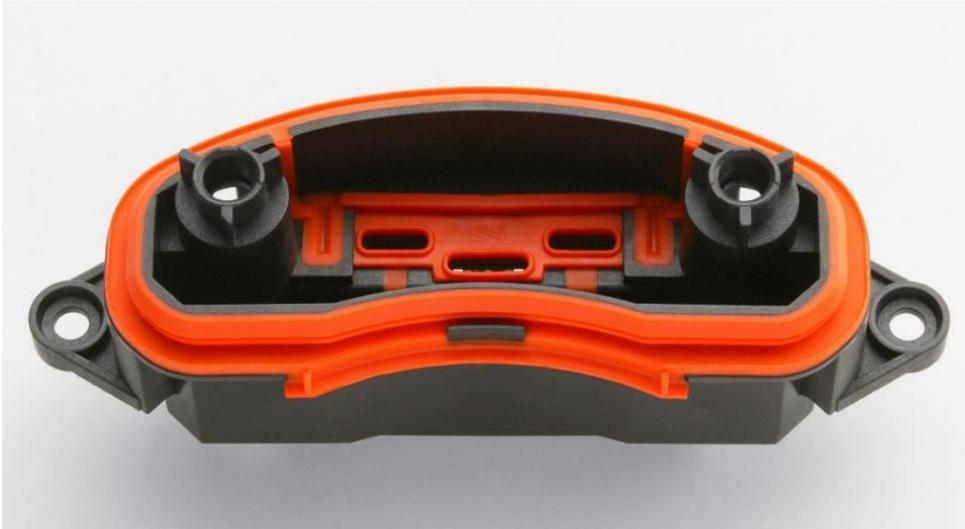
Connector housing with injection-molded orange radial seal made from ELASTOSIL® LR 3675. The self-adhesive liquid silicone rubber has a low-friction surface, which makes it easy to install. WACKER will be exhibiting the product for the first time at this year's plastics show K 2019. (Photo: WACKER)
