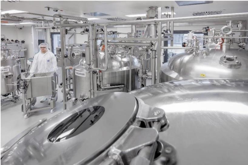
A cleanroom for producing biologics at WACKER's Jena site. Bacteria in the fermenters help produce active proteins for medications used, for example, to treat cancer and multiple sclerosis.
