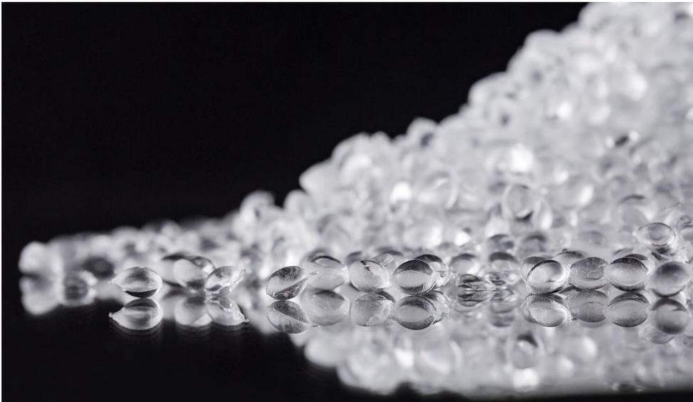
WACKER's new silicone additive GENIOPLAST® Pellet 345 lowers the hardness of thermoplastic polyurethane elastomers, while simultaneously boosting their surface properties. Plastic articles can thus be given a silky-soft surface that is resistant to abrasion and contamination. (Photo: WACKER)
