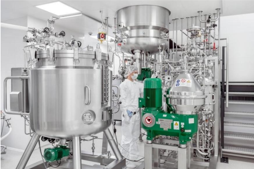
In stainless steel tanks known as fermenters, bacteria at Wacker Biotech produce the desired active substances (photo: WACKER).
