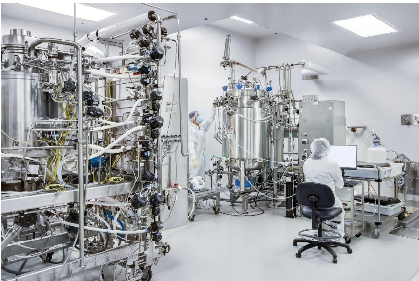
As a contract manufacturer, Wacker Biotech US Inc. in San Diego operates a specialized fermentation line for manufacturing and purifying plasmid DNA (photo: WACKER).
