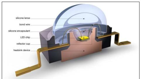
Section through an LED. LUMISIL<sup>®</sup> makes it possible to produce a moldless optical lens directly on an LED chip, using a dispensing process in a single production step. In this manner, LED components with silicone lenses can now be manufactured in very large quantities with comparatively modest plant and process investment. (Graphic: Wacker Chemie AG)
