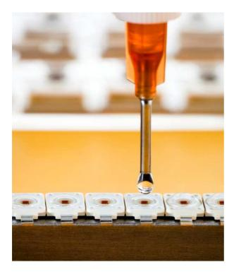
WACKER's new optical highperformance silicone brand LUMISIL<sup>®</sup> enables optical lenses for LEDs to be produced directly on the light-emitting diode chip. The process is highly efficient and cuts the traditionally high cost of LED production.
