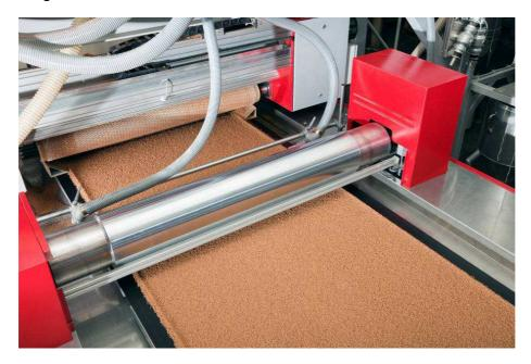
A machine known as a double-belt press is used to bond the cork layers to waferthin slate sheets under elevated pressure and temperatures of roughly 180 degrees Celsius (photo: Wacker Chemie AG).
