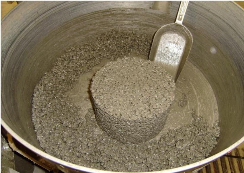
Freshly mixed drainage concrete in laboratory trials: the open-pored structure and pores can be clearly seen. Thanks to the new ETONIS® 260 polymer, the non-slump fresh concrete does not flow or disintegrate at the edges – this is a vital prerequisite for level track surfaces (photo: Wacker Chemie AG).
