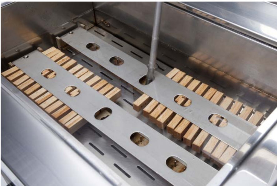
Conditioning of wood specimens according to DIN EN 204 for testing the shear strength of waterproof wood glues. (photo: Wacker Chemie AG).
