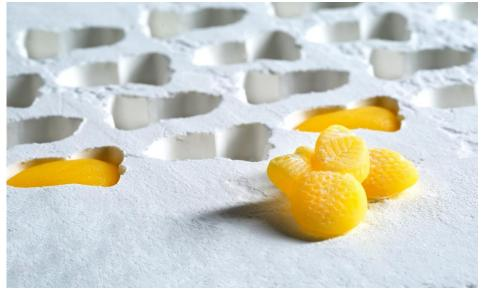
At ProSweets Cologne 2018, WACKER is introducing its new process for depositing sugar-free chewing gum to a wider specialist audience for the first time. Thanks to this new process, gum can now simply be molded into different shapes, similar to gummy bears (photo: Wacker Chemie AG/Bosch Makat Candy).
