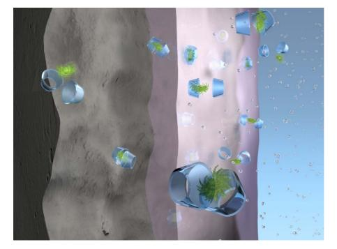
Model of cyclodextrin fragrance complexes in wall paints: The ringshaped sugar molecules can host fragrances in their inner cavity. Set off by moisture, they are released to their surrounding in a controlled manner (photo: Wacker Chemie AG).
