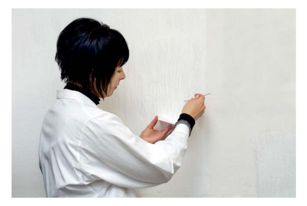
Taking a sample from a wall treated with a coating containing cyclodextrin fragrance complexes. By molecular inclusion in cyclodextrin, for the first time, essential oils and other fragrances can be used in plasters, paints and other coatings (photo: Wacker Chemie AG).
