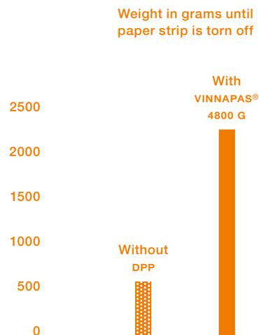
Joint fillers formulated with the new VINNAPAS® 4800 G gypsum binder offer greatly improved adhesion even to paper strips. The strips are often used to prevent cracks during the installation of plasterboard.
