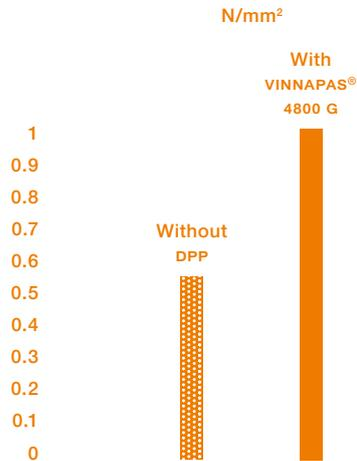
Comparative tests show that joint fillers formulated with the new VINNAPAS® 4800 G gypsum binder demonstrate much better adhesion than unmodified formulations.
