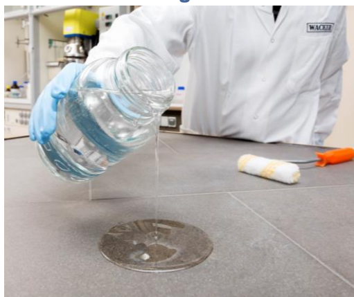
Protective Coating of Tiles
