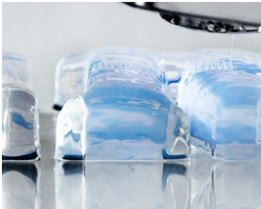
3D printing with silicones
