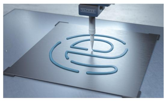
WACKER thermal adhesives are ideal for automotive e-mobility battery applications, thanks to their easy handling, pigmentability, and excellent mechanical properties. (Source: WACKER)
