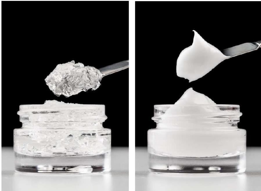
BELSIL® REG 1103 B silicone resin elastomer gel (left) becomes stiff cream (right) after mixing with water. (Photo: WACKER)
