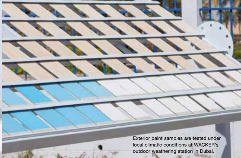
Exterior paint samples are tested under local climatic conditions at WACKER's outdoor weathering station in Dubai.
