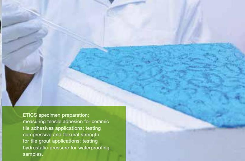
ETICS specimen preparation; measuring tensile adhesion for ceramic tile adhesives applications; testing compressive and flexural strength for tile grout applications; testing hydrostatic pressure for waterproofing samples.
