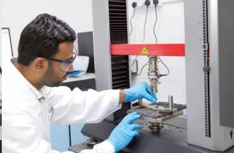
In the new carpet lab, a WACKER expert is conducting a tuft bind strength test.
